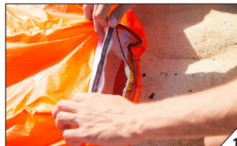
13 Close the Leading Edge air intake velcro.
