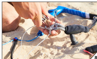
Wind the Trimmer Bracket screw back in.
