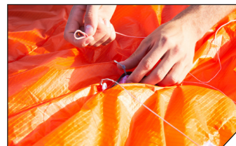
Connect the ISL line end to the internal knot using a larks head connection.
