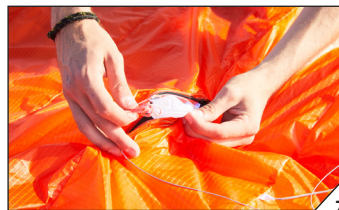
7 Pack the rest of the ISL line into the pocket on the rib (profile section)
