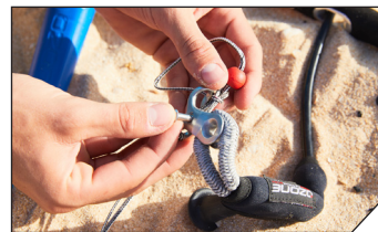
Pull line no.5 out through the Quick Release and bar centre.
