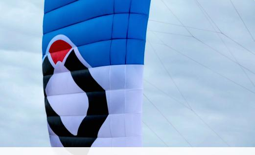
The Leading Edge now features Double Transversal Shaping creating a cleaner surface on the most important area of the aerofoil. The result is less turbulent airflow and longer skin adhesion, which positively effects the lift to drag ratio increasing overall performance.
