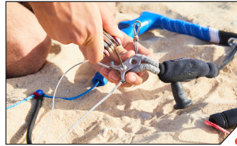
Remove the Trimmer Bracket screw.
