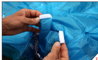
13 Reach inside the valve and undo the velcro retainers at the end of the valve sock on the left and right sides connecting to the ribs.
