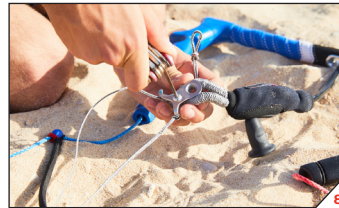
Wind the Trimmer Bracket screw back in.
