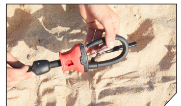
Unwind the first 3 metres of line no.5 from the plastic winder.
