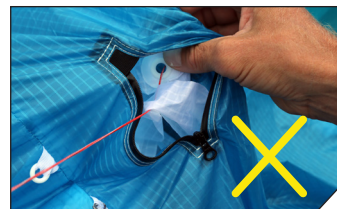
5 Ensure the ISL is not twisted around any structural parts (ribs/straps) inside the kite. The line should be running freely from the neighboring rib and out to the zip opening.
