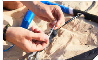
Undo the small line loop from line no.3. Store the small line loop.
