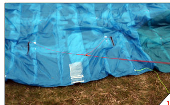
10 Ensure the connected LSL and ISL lines are running freely in between all Bridles and the Speed Systems.
