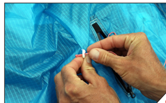
6 Feed the ISL line through the plastic ring on the bridle line tab next to the zip. Feed the line from the zip opening side towards the center.
