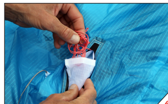
4 Open the pocket and take out the ISL line. Ensure there are no tangles or knots in the line.
