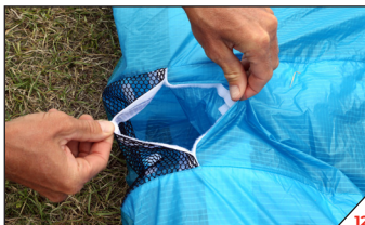
12 Open the Leading Edge air intake velcro to access the valve.
