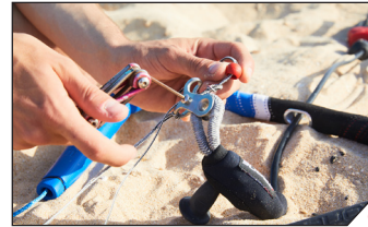
Remove the Trimmer Bracket screw.
