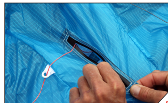
7 Close the zip until 5mm before the slider goes into the bungee cover, leaving room for the ISL line to run freely.
