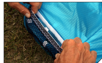
16 Fit the rolled valve inside the kite.
