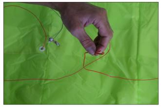
5: Guide the Internal Re-Ride Line through the Stainless steel ring. Repeat on the other side.
