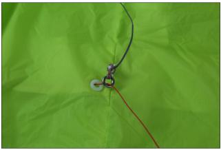
6. Connect the Internal Re-Ride Line back together with the riser line, and connect your 5th line back onto the pigtail and you are ready to go again!
